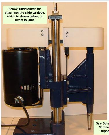
This undercutter is for handling large armatures in a lathe. It can be mounted directly on the lathe or on the Slide Carriage which bolts to the lathe cross-slide. The motor is 3/4 h.p. With gear-belt drive it has enough power and rigidity to use 7/8" O.D. x 5/16" I.D. Tungsten-Carbide Saws at 4600 r.p.m. By interchanging pulleys it will also use 7/8" O.D. x 5/16" I.D. High-Speed Steel Saws at 2600 r.p.m.
