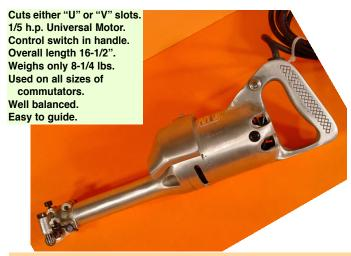
The model K Mica-Miller is an excellent all-around Undercutter for industrial plants or repair shops, as it can be used in the shop or taken to the job, and can be operated on A.C. from any lighting circuit.
