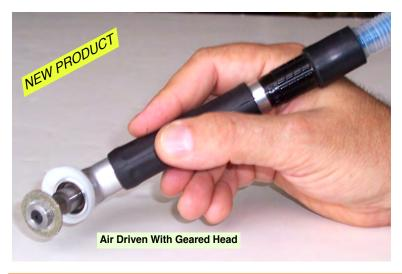
The Mini Kut-Kwik is a compact, high speed (35,000 R.P.M.) air operated undercutter, ideal for use in confined spaces where a standard sized hand held undercutter would be too large. The high-speed allows use of diamond plated wheels for a smooth cutting action. Although this tool can be used continuously on an undercutting operation, it is not intended for heavy cutting.
